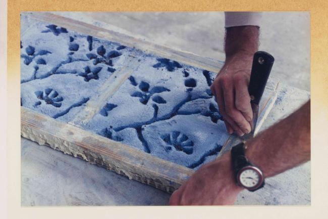
excess blue cement is scraped off frames and blown clean with compressed air.
