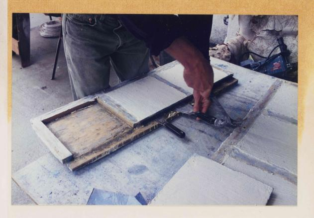
each tile is carefully removed from the remainder of the frame.
