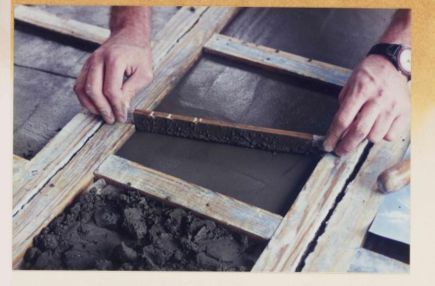
each tile is screeded off to a common depth.
