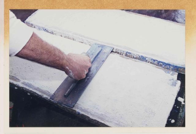
the white layer is troweled off even with the edge of the frame.
