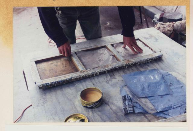
the process begins with the waxing of pre-made frames to allow for easier removal of the tiles. sheets of plastic also aid in keeping the bond between the frame and tile.
