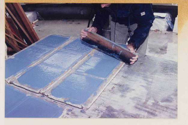
each frame is vibrated by hand to allow air bubbles to rise and escape.
