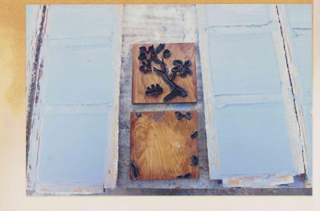
the tiles are allowed to set for 10-20 minutes until the blue cement is stiff enough to hold the imprint of the pattern cutters.
