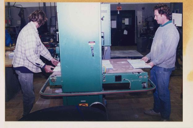
at the shop, tiles are passed through a time-saver equipped with a belt specifically designed for grinding cement.
