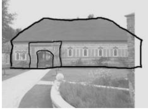
Figure 21: Within the overall building 'center', the entry porch is the strongest 'center', achieved in large part by the darkness of the actual doors contrasted with the surrounding mass of the porch (see Contrast below).
