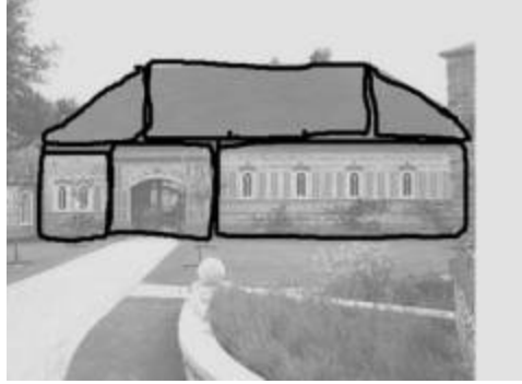
Figure 15: Roof mass divided into area under ridge, approximately \frac{3}{5} and area of hips, approximately \frac{1}{5} each, somewhat weak. Facade divided into right hand portion, approximately \frac{3}{5} and projecting entry porch, approximately \frac{1}{5} and left hand portion, approximately \frac{1}{5} .
