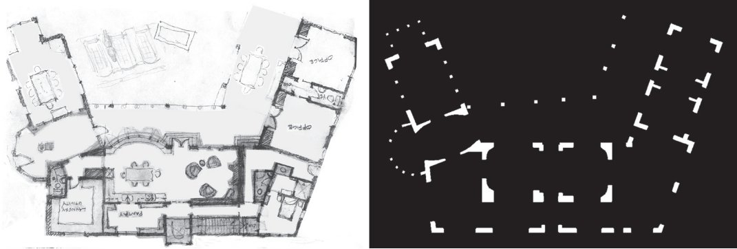
Step 6: The plan of the Sanders house, as it emerges from the previous differentiations through the action of the BOUNDARY transformation, supplemented by the action of LEVELS-OF-SCALE, STRONG-CENTERS, LOCAL-SYMMETRIES and ROUGHNESS transformations. Step 7: The right hand drawing shows the structural plan which emerged from this plan shortly afterwards.
