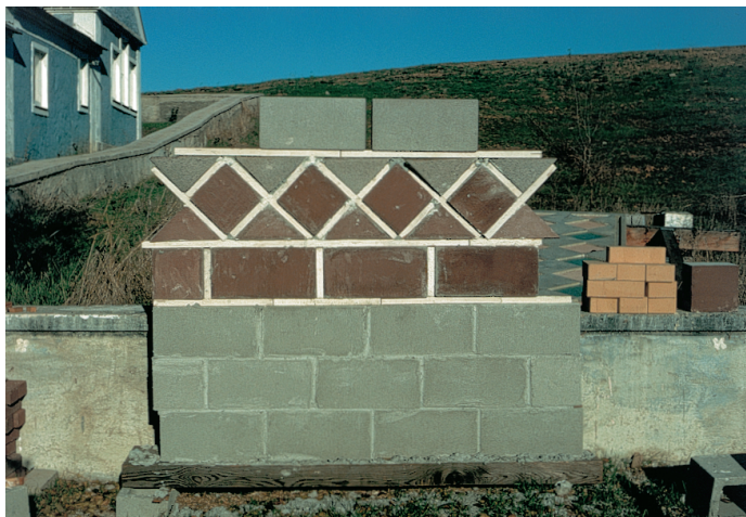
Another experiment trying a combination of red pavers, white plaster strips, brick, concrete, and concrete block
