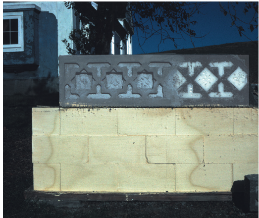
First mockup of poured concrete shapes with cement plaster and styrofoam insets
