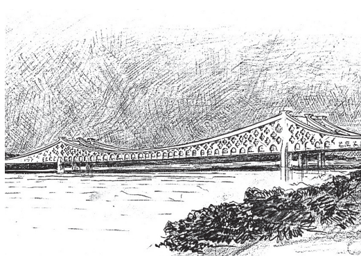
The Puerto Rico Bridge, prestressed concrete shell design, 500 meter span, by Center for Environmental Structure and T. Y. Lin International, 1995
