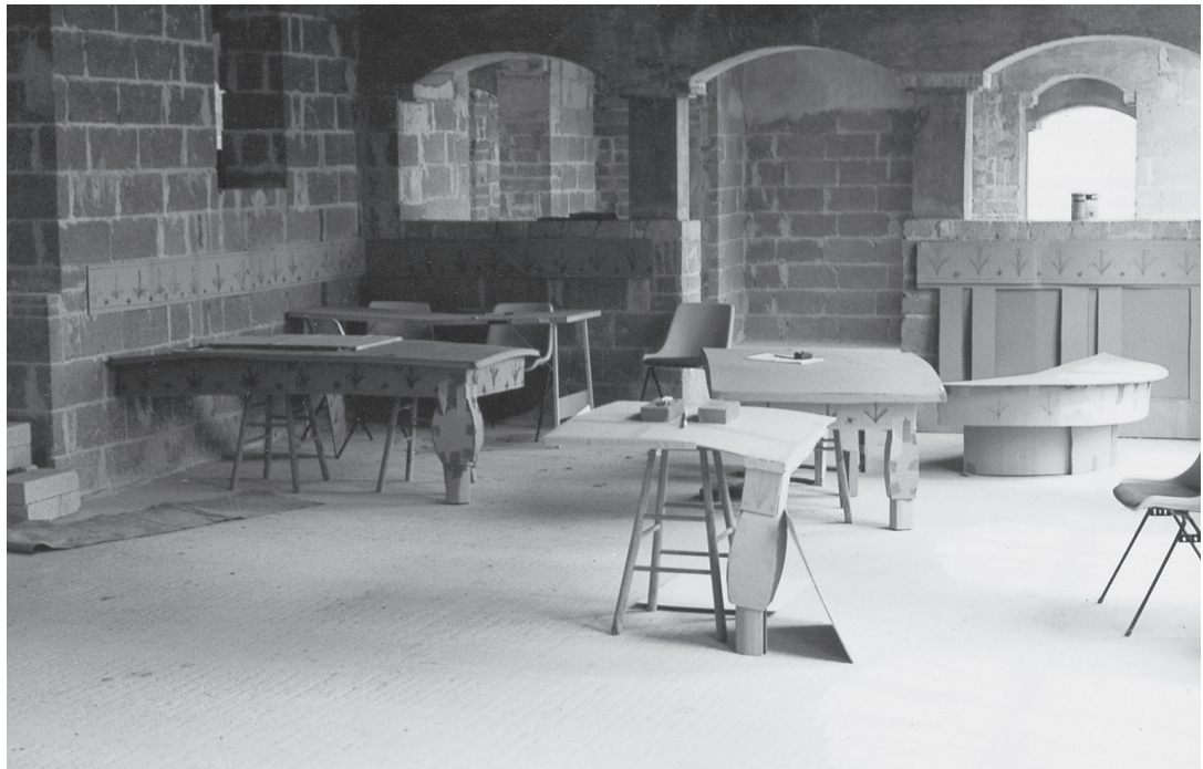
Early cardboard and wooden mock-ups of the furniture we were designing for the building. After reconciling the feeling of the furniture with the actual place while it was still in construction, we then built the tables and chairs according to these mock-ups.
