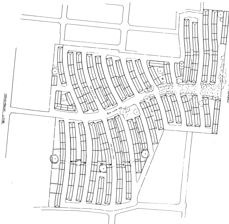
Shiratori Housing, Nagoya. Five hundred apartments on 2.5 hectares. Christopher Alexander and Miyoko Tsutsui, 1988.
