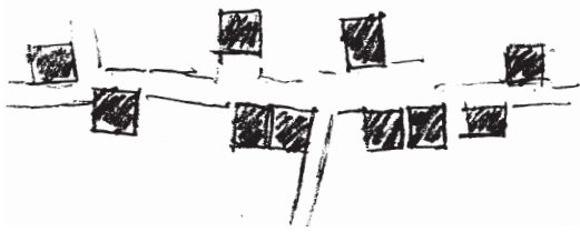
Step 4: House positions placed (before lots) to form and shape the perimeter of a street volume.
