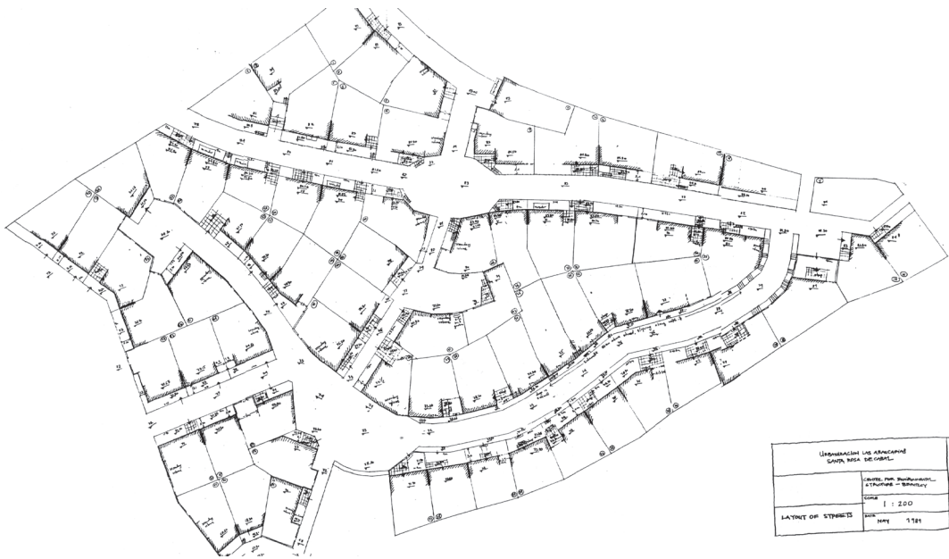
Lot plan, showing the seventy lots laid out on the site. This drawing reflects the results of work on the neighborhood layout and streets, by CES staff with seventy families. It is additionally described in chapter 9.
