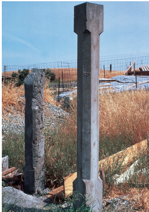
A sample gunite column, shaped to be beautiful and easily formed by the open-form technique.
