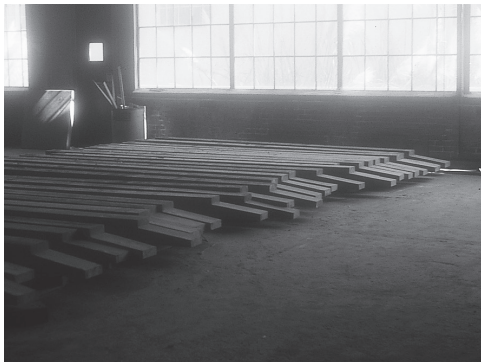
Freshly prepared columns in our shop, waiting to be put on the truck and taken to the site.
