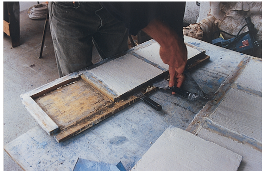
Removing tiles from forms
