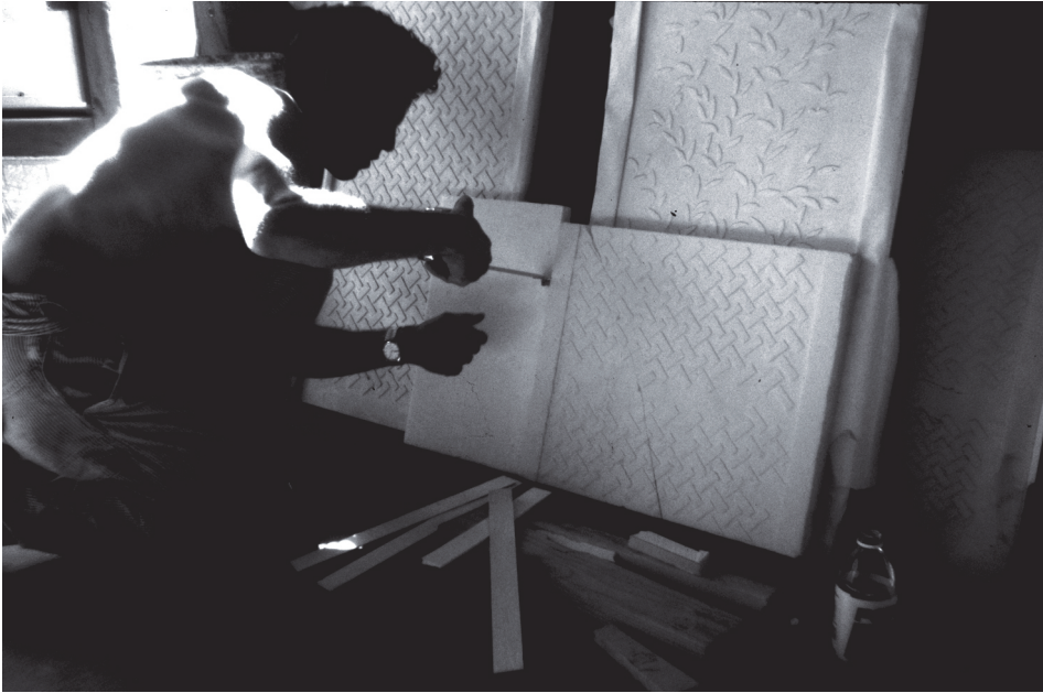
Randy checking widths, details of the edge band on the plaster panels of another project. On these panels, it turned out that a difference between 1/8, 1/4, and 3/8 of an inch in thickness was of tremendous significance.
