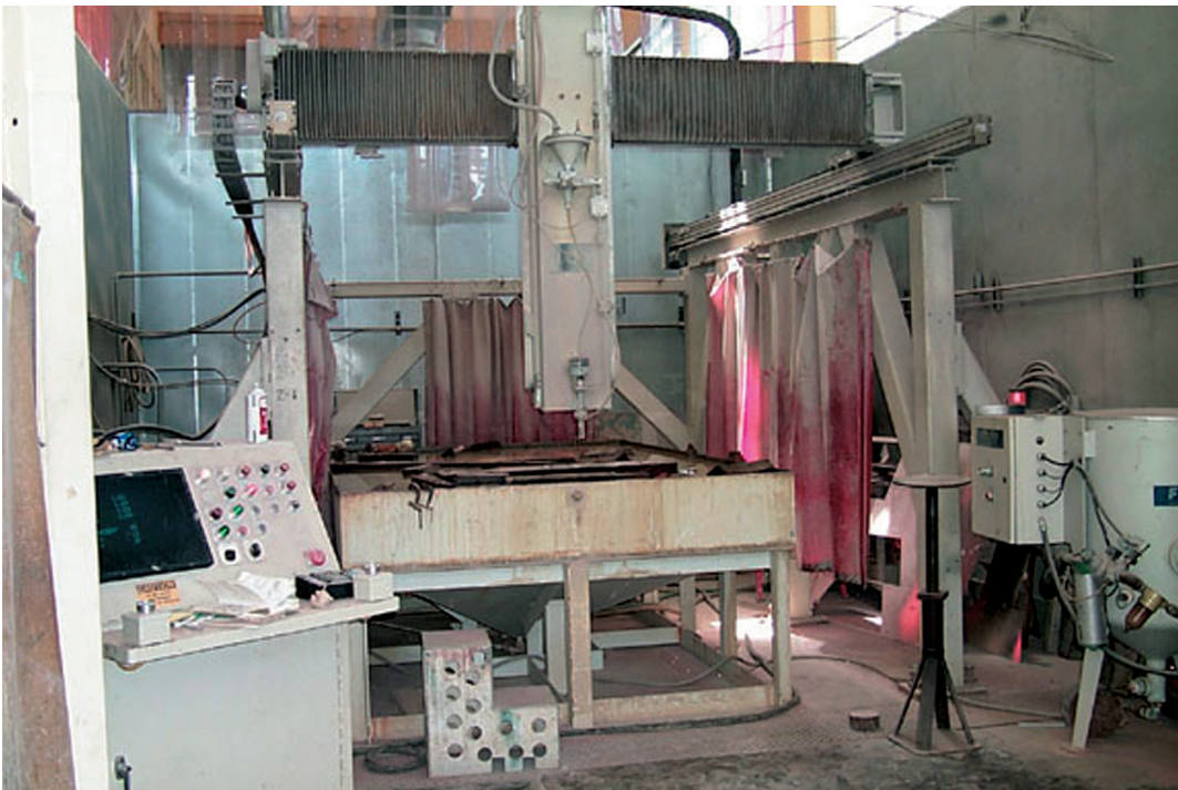
A computer-controlled water-jet cutter in Germany
