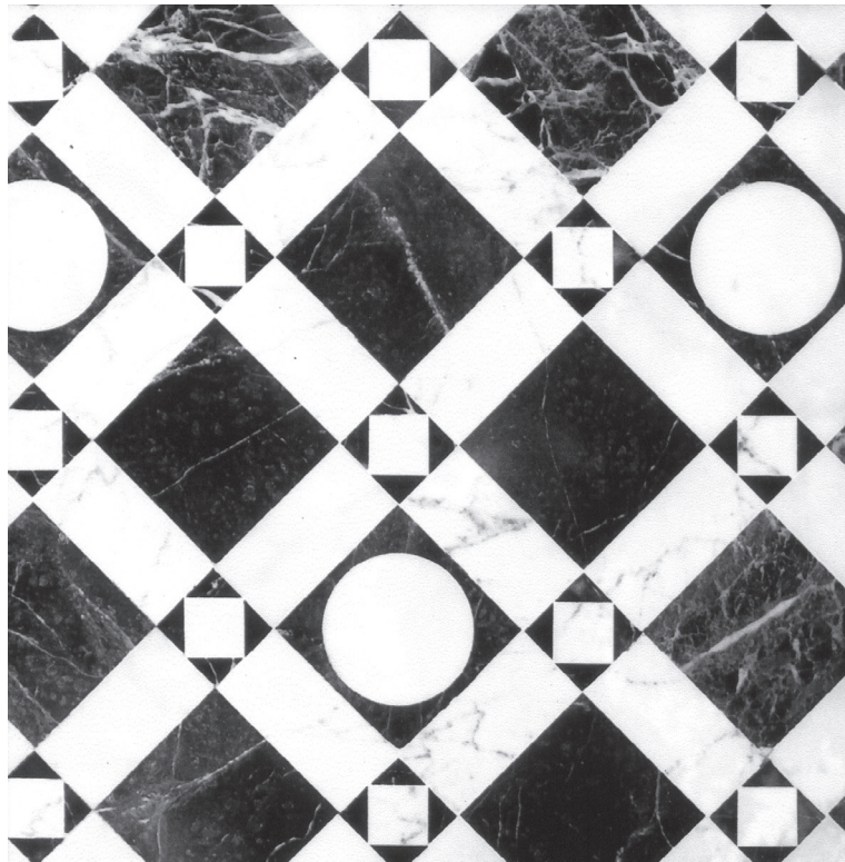
A small piece of a floor, in black, white and green marble, sketched and designed by the full-size mockup techniques described on pages 566–70. This sample is about 18 inches by 18 inches, contains 100 pieces, the smallest less than an inch across. It was laid out in CAD from our rough sketches, then cut and fabricated in about an hour.
