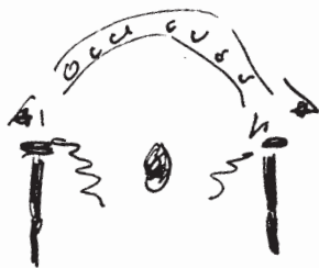
First sketch of deep pile foundations on either side of the dry dock, to carry the arched trusses without loading or damaging the weak stonework of the ancient dock construction.
