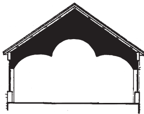
4b. Our final definition of the truss envelope, showing cross-sectional shape with main arch and two half arches
