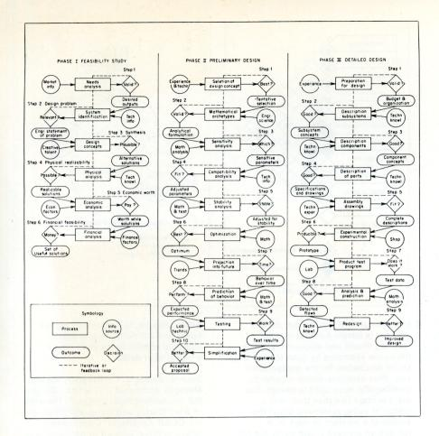
3 A typical attempt to plot the design process using the symbols of computer programming, from Asimow. Most designers believe, quite rightly, that their brains cannot operate efficiently to such a rigid schedule and Asimow's description of this as a design 'morphology' introduces a piece of unnecessary jargon. Design 'process' would be a perfectly adequate term for it.
