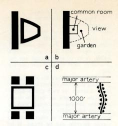
6 The solution to each subset of Alexander's misfit variables is represented by means of a diagram. Here are the first four of twelve such diagrams by which he 'solves' the problem of urban loneliness by clustering the various parts of a house around a communal 'fish tank', into which people can see from the street. You are supposed to sit there, in full view of passers-by, whenever you feel lonely and want people to call on you.
