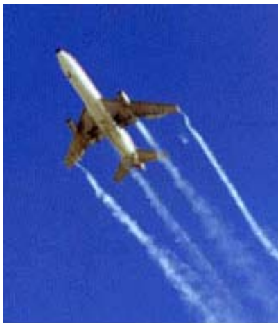
Figure 22b. The cylinders of vortices seen as two outer parallel trails emanating from the wing tips. (The inner trails come from the engines.) (From [36])
