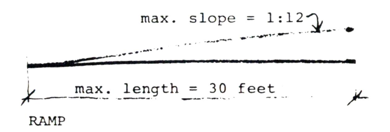
Therefore: Put ramps, with maximum slopes of 1 in 12, or elevators, at least 5 feet square, in every public place or building with a change of level, so that all public parts of the place or building are open to the old and handicapped.
