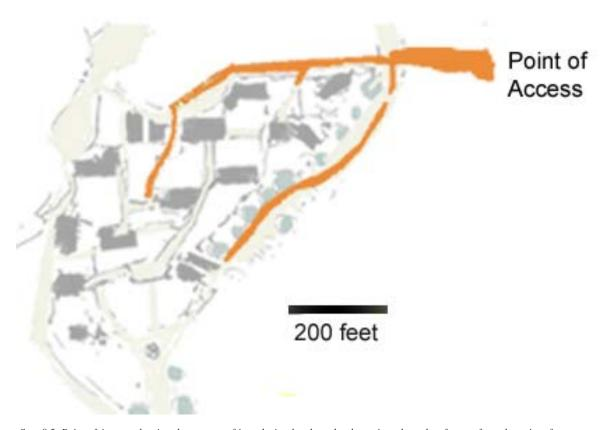
Step 8.5. Point of Access, showing the process of introducing local roads, shown in red, as they fan out from the point of access. The black bar shows the dimension of 200 feet, and allows one to see that in this neighborhood, only two houses (as permitted) are more than 200 feet from the local roadway.
