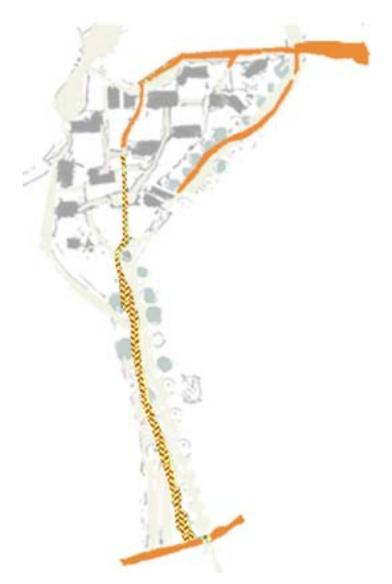
Step 8.6. The process of introducing a secondary loop of pedestrian hard paved surface capable of taking fire trucks and other emergency vehicles.
