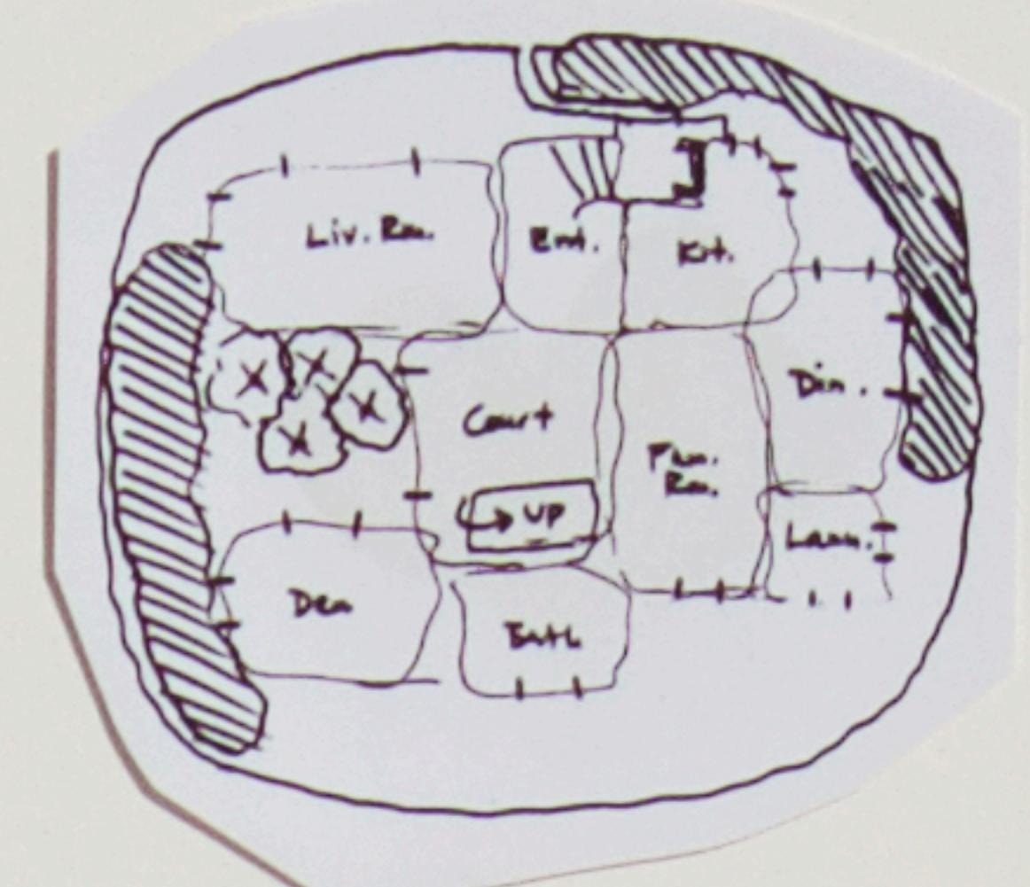
Towards the end of the house design process, the family will put the construction into their previous design decisions. One example of a structural pattern has to do with the placement of wooden columns in post-and-beam construction used in California. Columns at the corners explains how one begins to give structure to the design by placing columns at the corners of all social spaces, then continuing to add other columns along their sides to form structurally sound bays.
